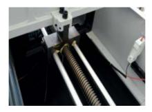
Pull out the front covering strip, and cheak stepping motor, to see whether the synchronous pulley and synchronous belt are fixed normally;
