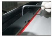
Tighten screws on blade carrier, Put on the up cover, then fix up;
