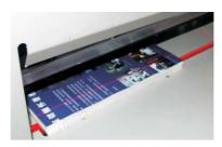
Turn the protective switch to ON position. Screen display will be light and the lindicative line light on the machine will be bright. The machine can be operated after backgauge is cailbrated automatically.
