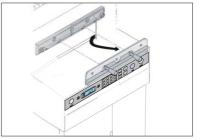
When you install the blade, you should screw up the screwstems. Insatall the blade on the blade carrier and use screw strip to fasten and fix up, then adjust accrding to cutting depth adjustment method;
