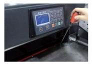
Note: When kinfe shim is being changed, the blade itself also needs to be adjusted. If the blade cuts too deep, the knife will be damaged easily, and the blade also will abrade rapidly.
