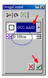
9. There are three types of GCC AASII registration marks: 4-Point Positioning, Segmental Positioning, and Multiple Copies. To make 'Segmental Positioning' marks, please select "GCC
