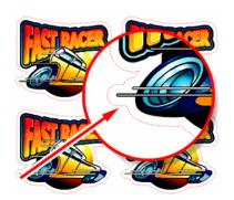
When your design is successfully imported into EasySIGN, you should then select the line or lines that you want to cut on your plotter. After selecting them, use the command "Edit, Convert to, Line type, Print&cut line". The lines that will be cut are now shown in a dotted red line. Copy the design as you like.
