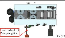
When bind thicker book, it may pre-open (smaller than block's thickness) guide wheel (only K9), to decrease impact force, lengthen machine's life.(this function also auto measure block thickness and guide wheel opening width)
